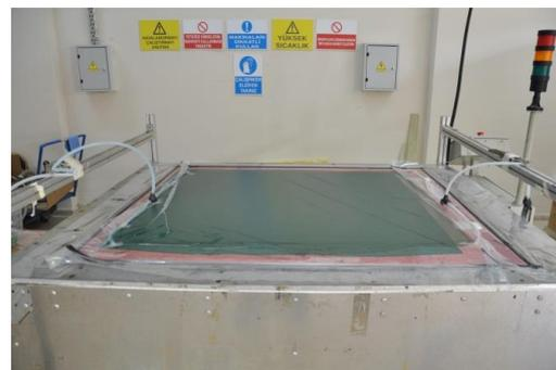
**Figure 1:** Vacuum Assisted Resin Infusion Molding Process
