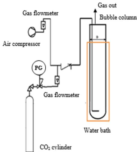
**Figure 3:** Lab-Scale batch of bubble column experimental Set-up
