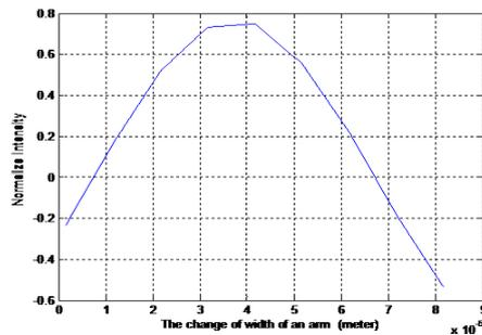
**Figure 12:** The change of the width( $\Delta w$ ) of an arm verses of normalize intensity
