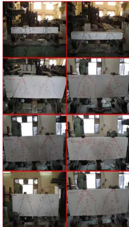
**Figure 9:** Cracking Patterns of the Tested Beams
