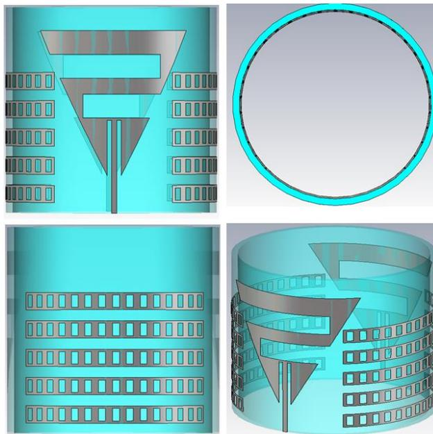
**Fig 2:** The antenna elements separated with MTM structures.
