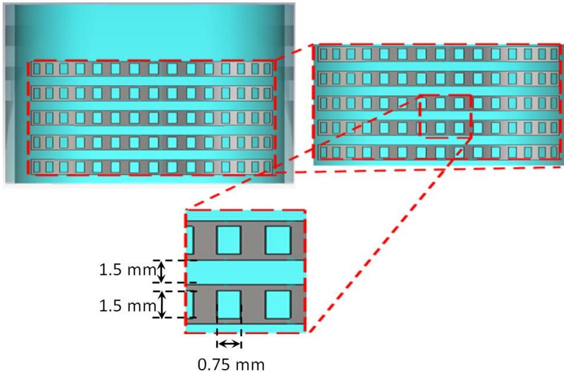
**Fig 3:** The periodical structure of single unit cell of the proposed MTM.
