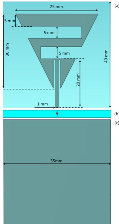
**Fig 1:** Single antenna structure: (a) front view, (b) side view, (c) back view.
