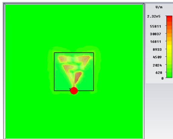
**Fig 8:** The electric field on the patch.
