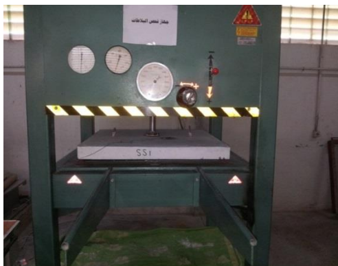
Figure (3) Test setup of solid and bubbled RC slab
