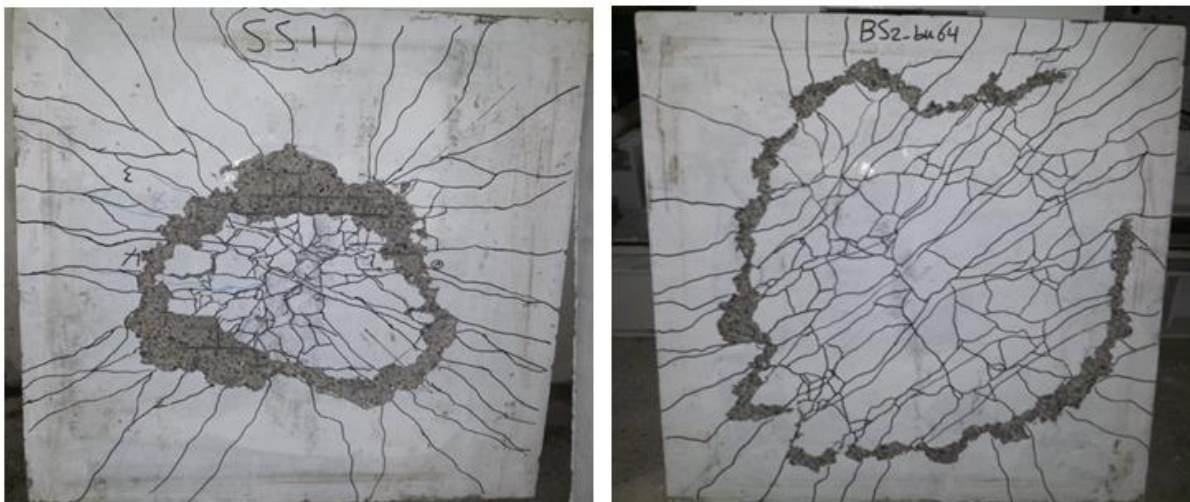
Figure (13) Crack patterns of slabs in group B (bottom face)
