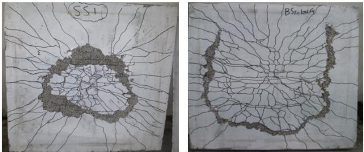
Figure (9): Crack patterns of slabs in group A (bottom face)
