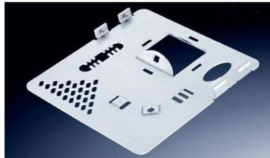
**Figure (2):** gasket and sheet metal perforation [Ref.]
