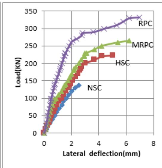
Fig.(9) Lateral deflection for panels with slenderness ratio ( $H/t=14$ ), ( $t=50$ mm)
