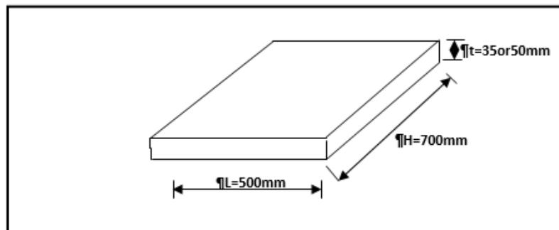
Fig. (1) Dimensions of wall panel
