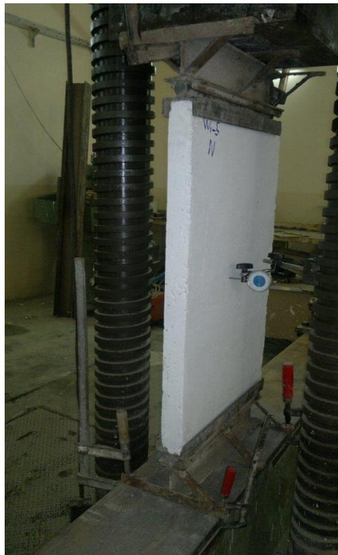
Fig. (2b) tested panel with the simply supported edges
