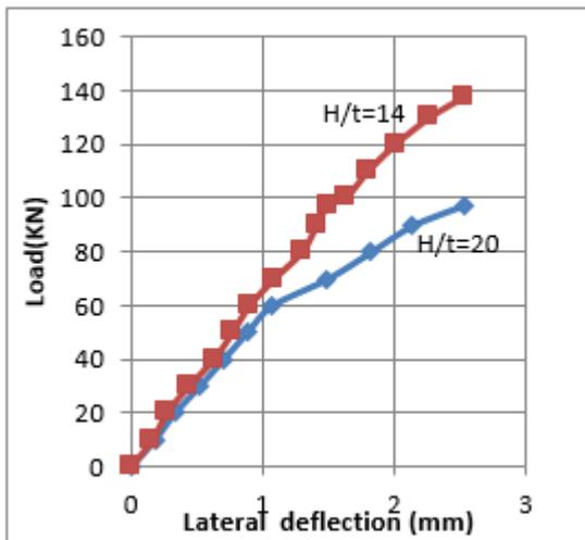
Fig.(4) Lateral deflection for panels with normal strength concrete ( $f_c=30.2\text{Mpa}$ )
