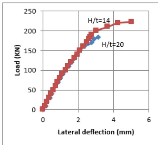
Fig.(5) Lateral deflection for panels with high strength concrete ( $f_c=69.5\text{Mpa}$ )
