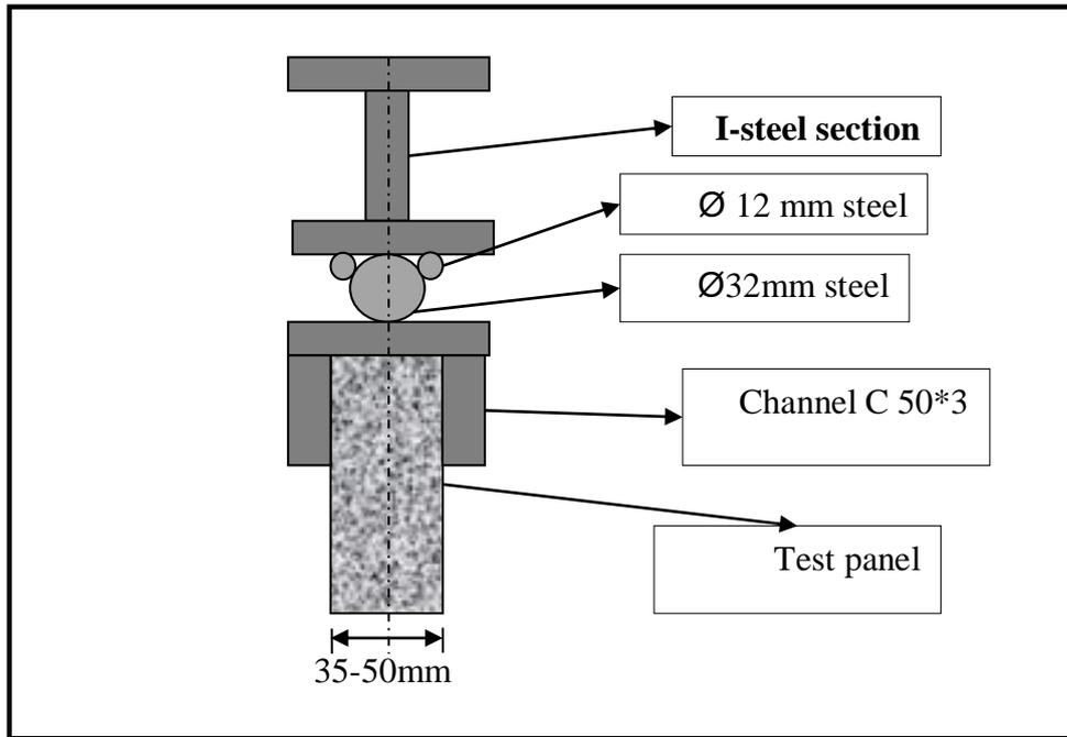
Fig. (2a) Detail of Supports used in this work
