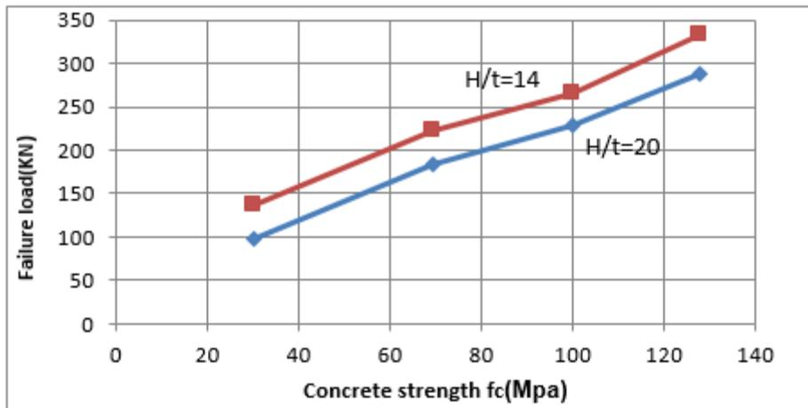
Fig. (10) Effect of concrete strength  $f_c$  on failure load for panels with normal, high strength, MRPC and RPC
