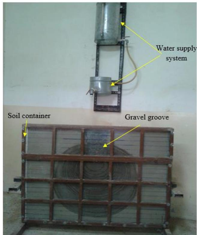
Figure (1). Layout of the soil container and the water supply system.
