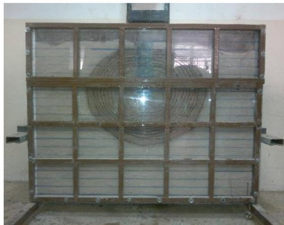
Figure (3). Shape of the wetting front pattern for  $q=1.3$  l/hr and  $w = 10$ cm.
