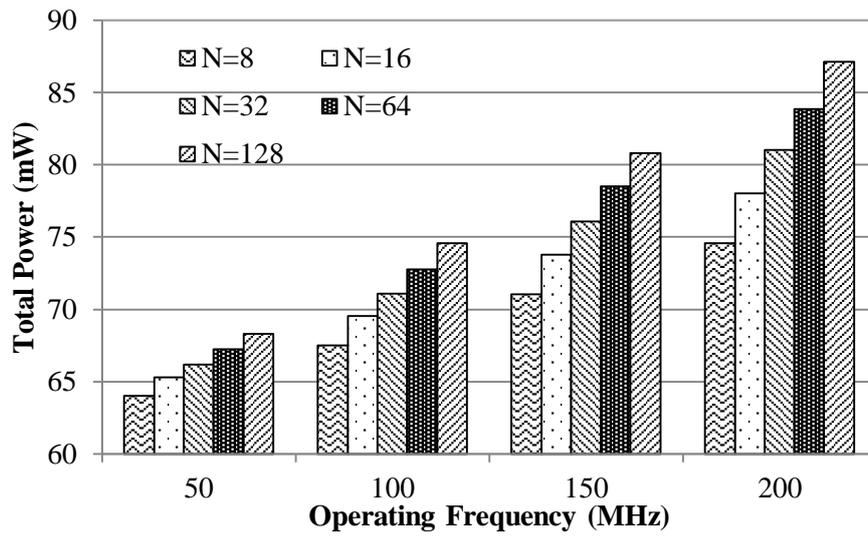
Figure (6): Dynamic power consumption of the proposed architecture using N=8, 16, 32, 64 and 128 for various operating frequencies
