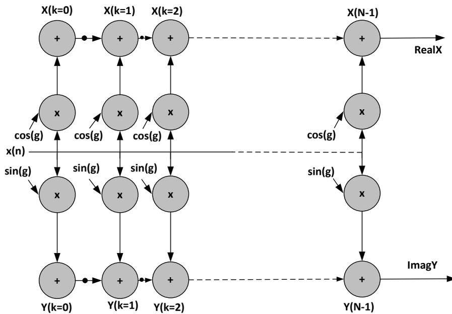
Figure (3): Synchronous Dataflow Graph (SDFG)
