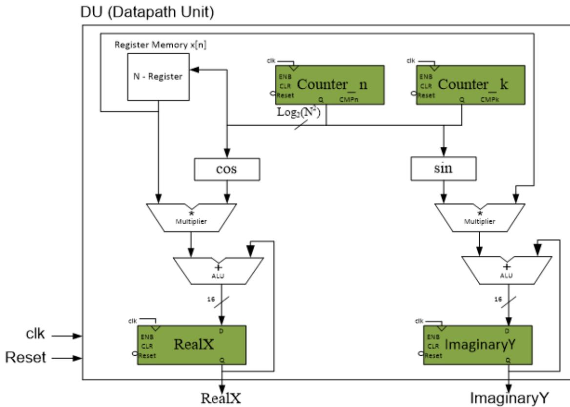
Figure (4): The Datapath Unit of the DFT.
