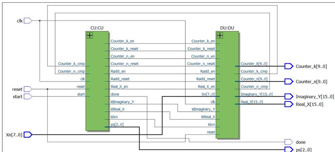
Figure (5): The Toplevel of DFT architecture for N=32
