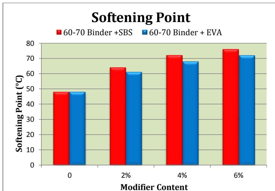
Figure 2: Softening Point Values of Modified and Natural Asphalt Cement
