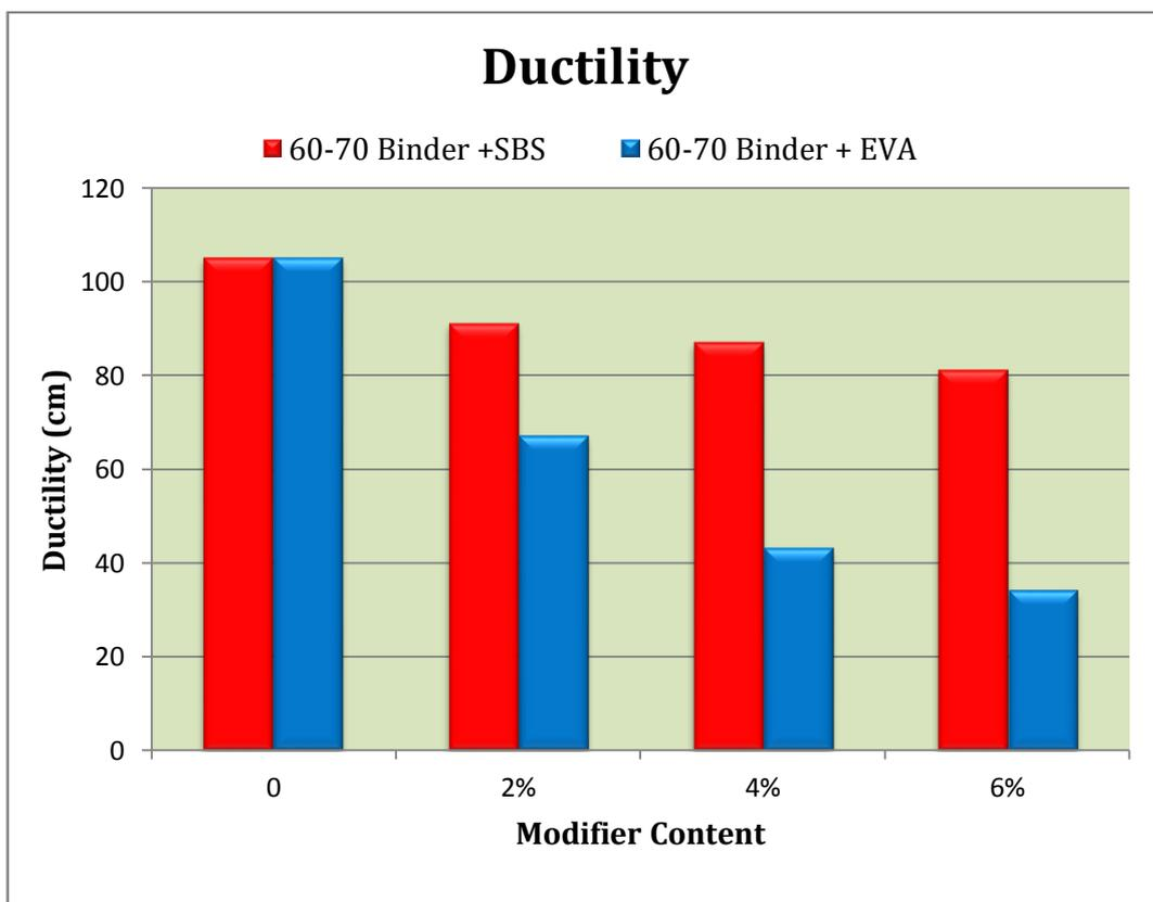
Figure 4: Ductility Values of Modified and Natural Asphalt Cement
