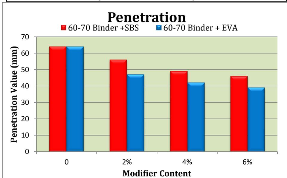
Figure 1: Penetration Values of Modified and Natural Asphalt Cement
