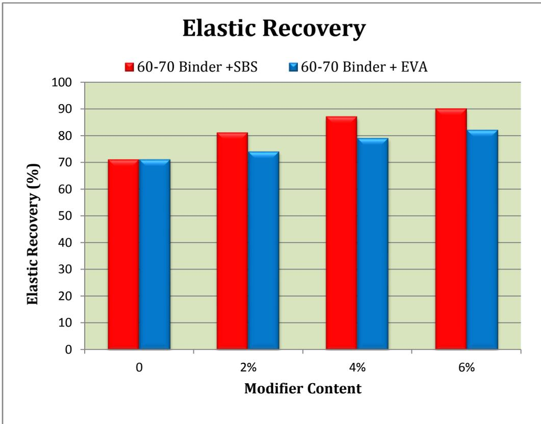
Figure 5: Elastic Recover Values of Modified and Natural Asphalt Cement
