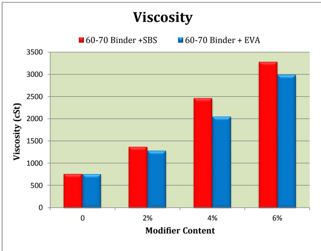
Figure 3: Viscosity Values of Modified and Natural Asphalt Cement
