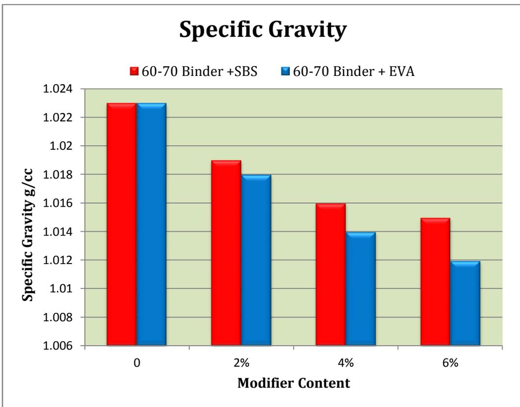
Figure 6: Specific Gravity Values of Modified and Natural Asphalt Cement
