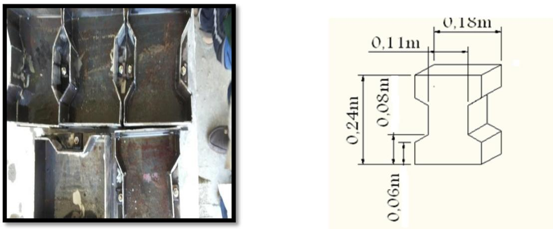
Figure (2) Molds and dimensions of concrete paving bricks.
