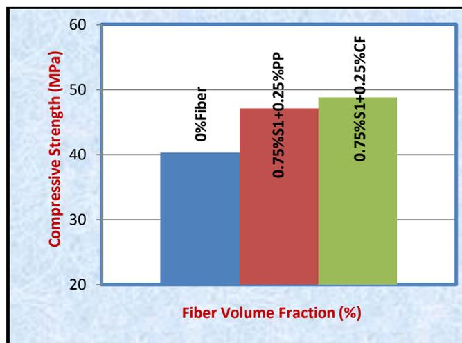
Figure (5) The Compressive strength of concrete paving bricks.
