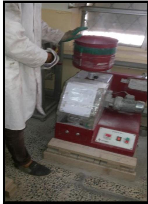
Figure (4) Abrasion resistance test for concrete paving bricks.
