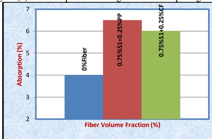
Figure (6) Absorption values of concrete paving bricks.
