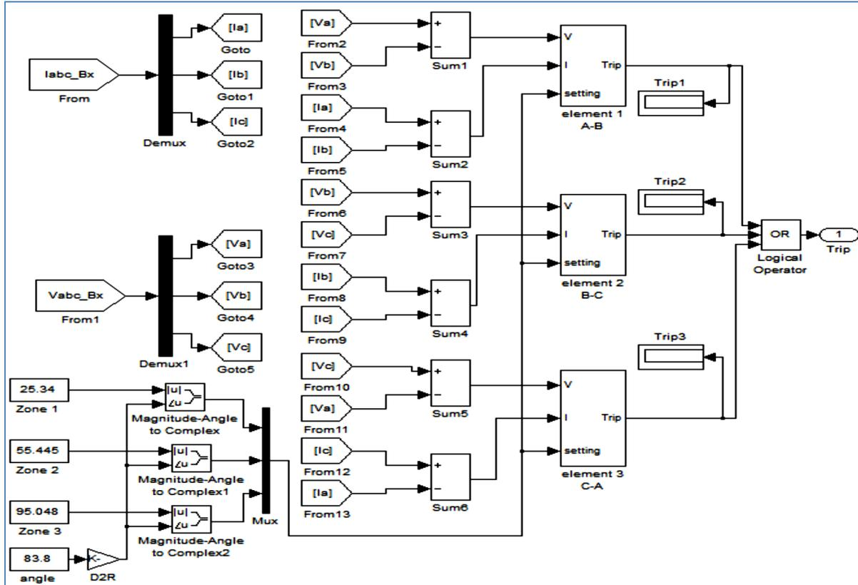
Figure (4) SIMULINK phase mho relay model
