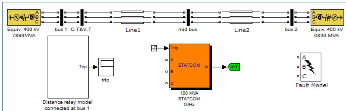
Figure (6) overall Matlab/Simulink system model
