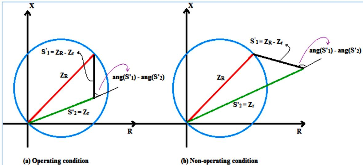
Figure (3) Sample Mho-relay characteristics
