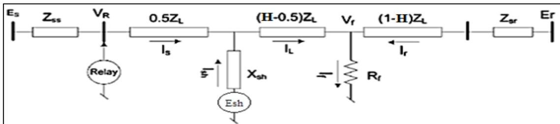
Figure (5) Simplified faulted network for a power system with STATCOM device
