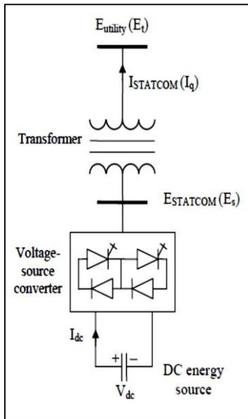
Figure (1) A STATCOM device circuit diagram [7]
