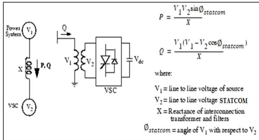
Figure (2) Operation principles of a STATCOM [8]
