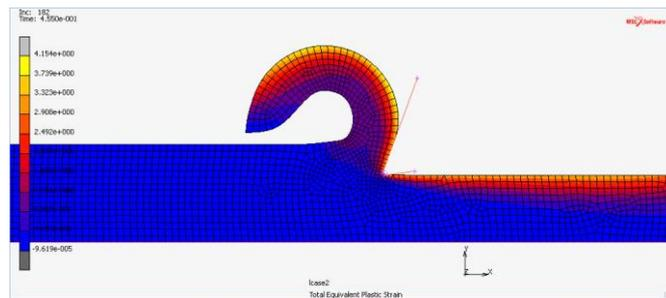
Fig. (3) Equivalent plastic strain case of 20° rack angle and 0.048 mm/rev feed
