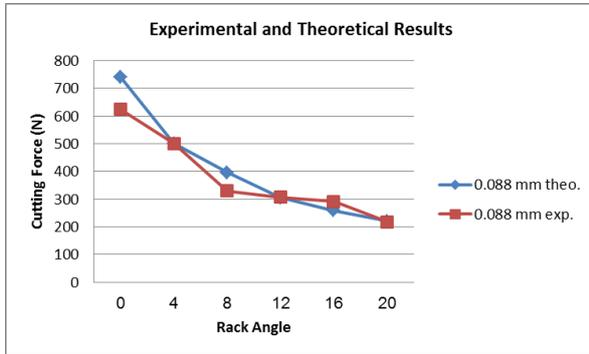
**Fig.(8) Comparison of current results with experimental results of Ref.(7) at 0.088 mm feed**
