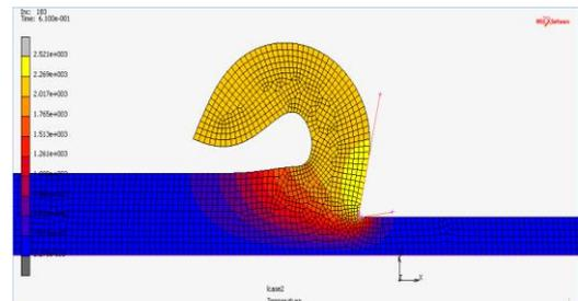
Fig. (2) Temperature distribution for case of 12° rack angle and 0.108 mm/rev feed
