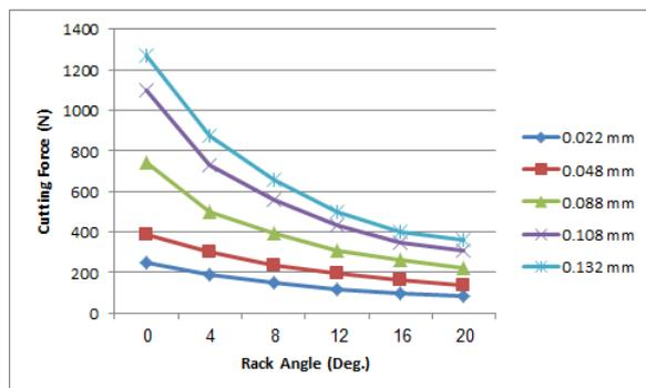
Fig.(4) Effect of rack angle on cutting force under different cutting feeds
