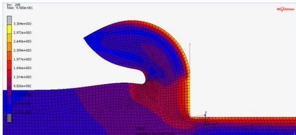
Fig. (1) Von Mises stress for case of 0° rack angle and 0.088 mm/rev feed
