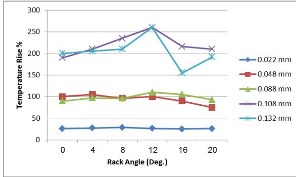
**Fig.(6) Effect of rack angle on temperature rise under different cutting feeds**
