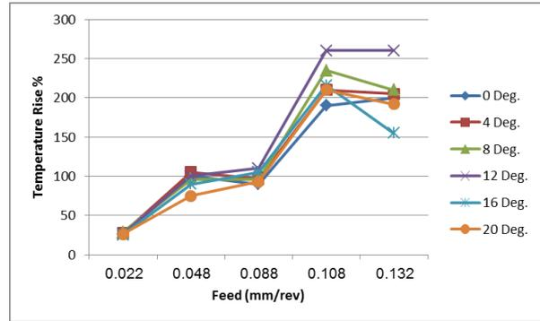
**Fig.(7) Effect of cutting feeds on temperature rise under different rack angles**
