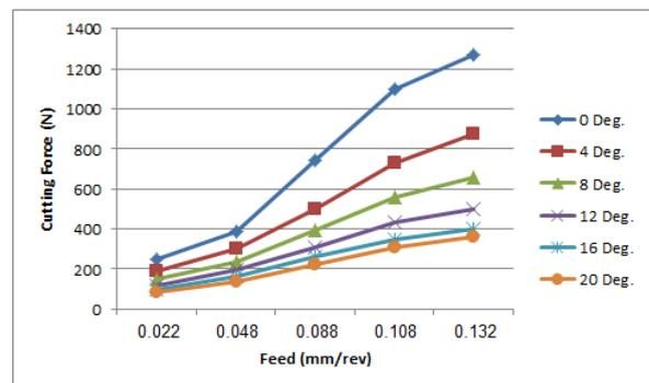
Fig.(5) Effect of cutting feeds on cutting force under different rack angles
