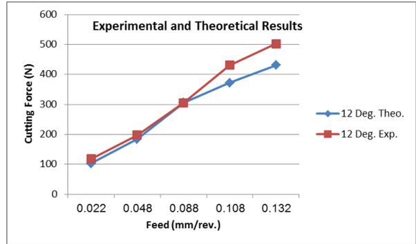
**Fig.(9) Comparison of current results with experimental results of Ref.(7) at 12° rack angle**
