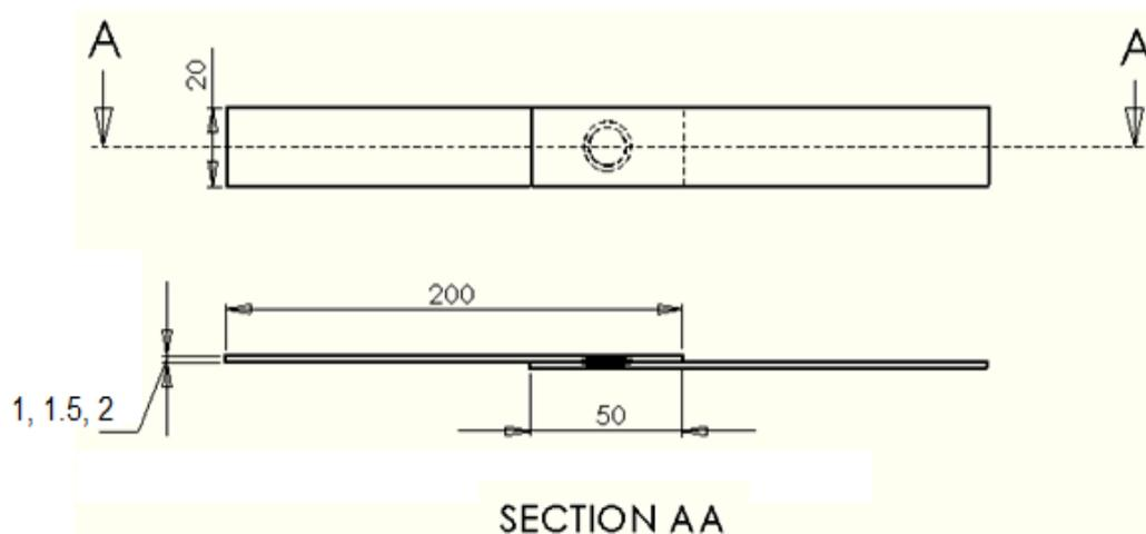
Fig. (2) Dimensions of the steel Sheet specimens
