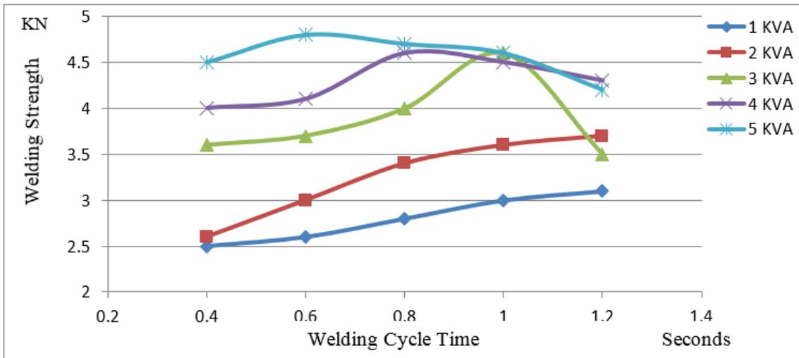
Fig. (3) Relation between welding time and welding strength for sheet thickness (1 mm)
