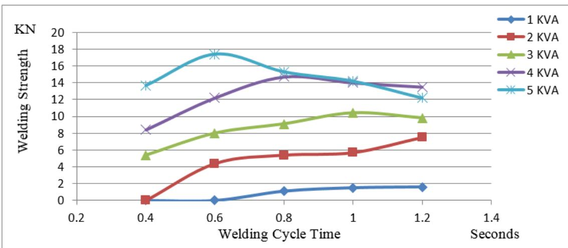
Fig. (5) Relation between welding time and welding strength for sheet thickness (2 mm)
