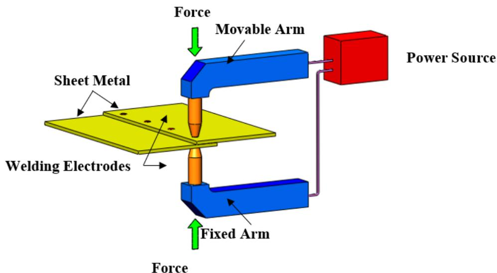
Fig. (1) Resistance Spot Welding
