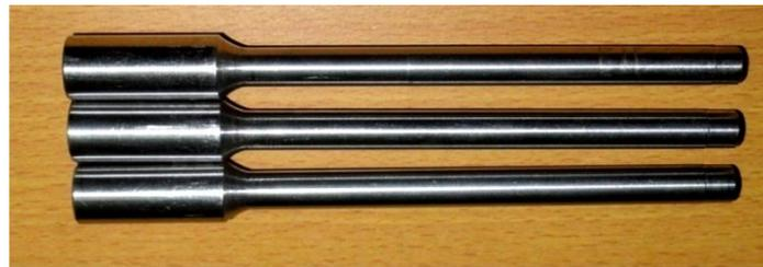
Fig.1 photograph of fatigue specimens
