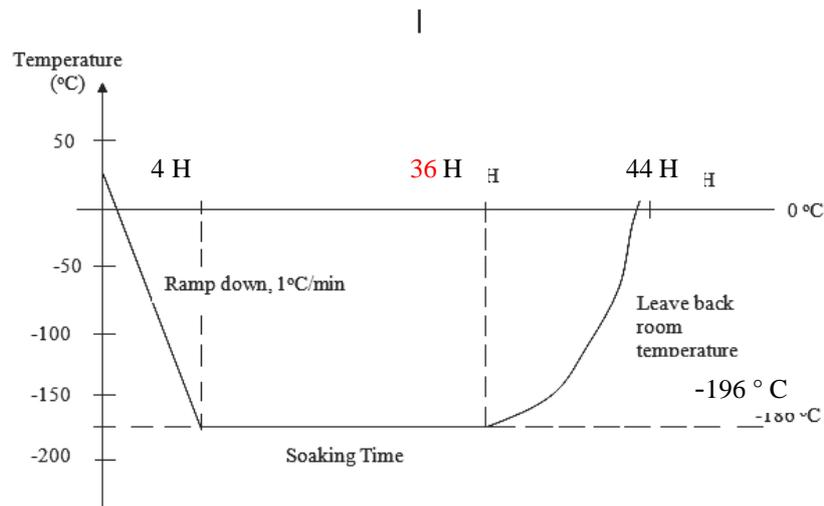
Fig.3 a typical cryogenic treatment for 17Mn4 steels.
