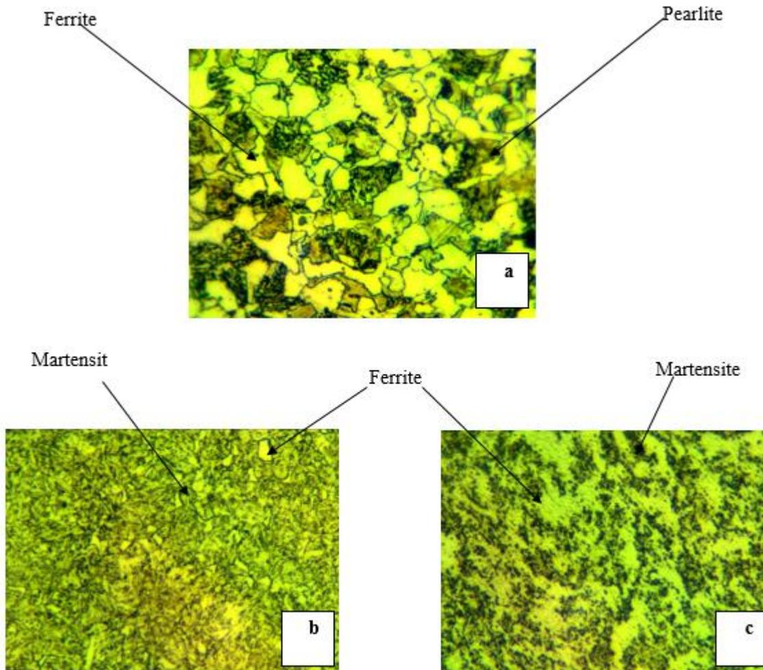
Figure 7 shows the microstructure of **a**-normalized steel **b**-ferritic-martensitic steel before **c**-after cryogenic treatment.
