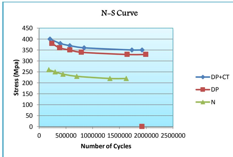
Fig.4 fatigue limits before and after cryogenic treatment
