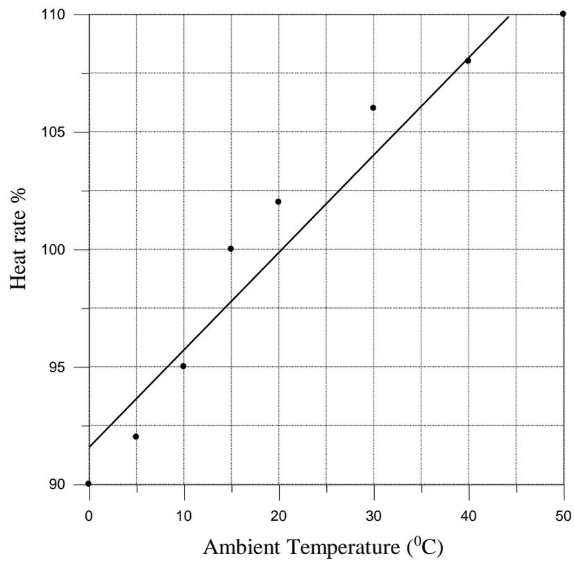
**Figure (5)** Ambient Temperature versus heat rate
