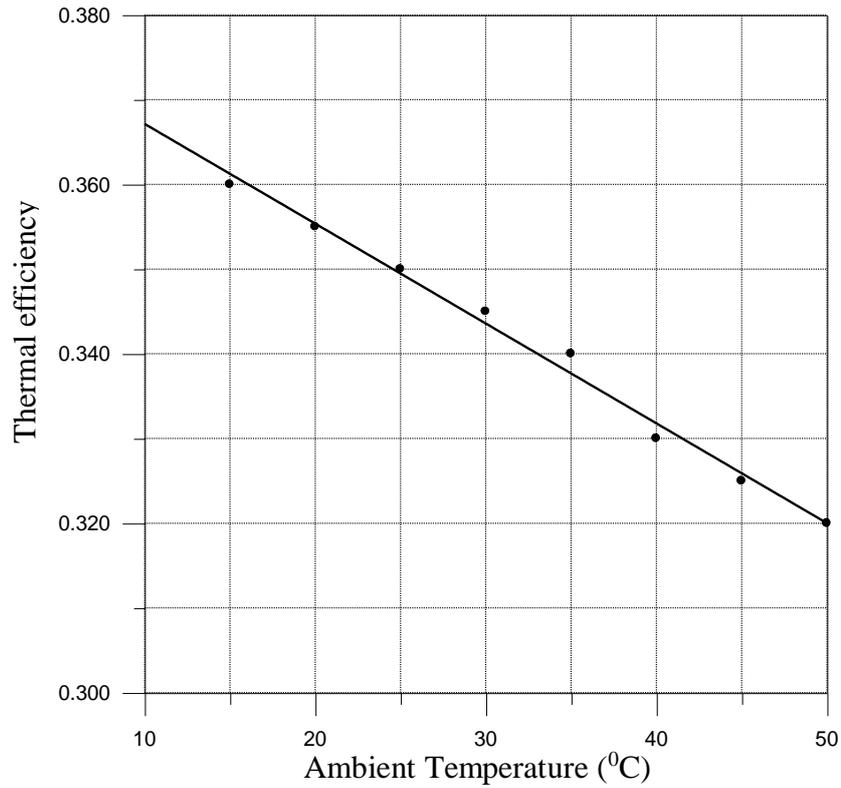
**Figure (8):**Ambient Temperature versus Thermal efficiency
