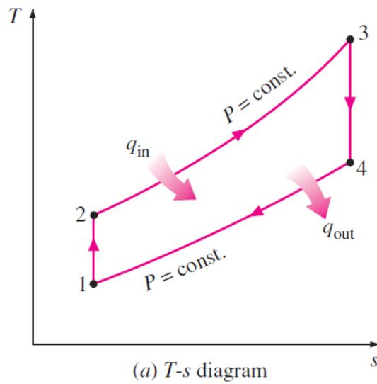
**Figure (2):** Brayton cycle of simple gas turbine power plant on T-S diagram
