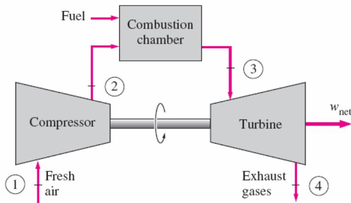
**Figure (1):** Simple open gas turbine power plant
