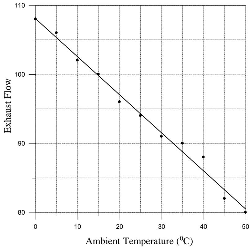
**Figure (7):** Ambient Temperature versus Exhaust Flow
