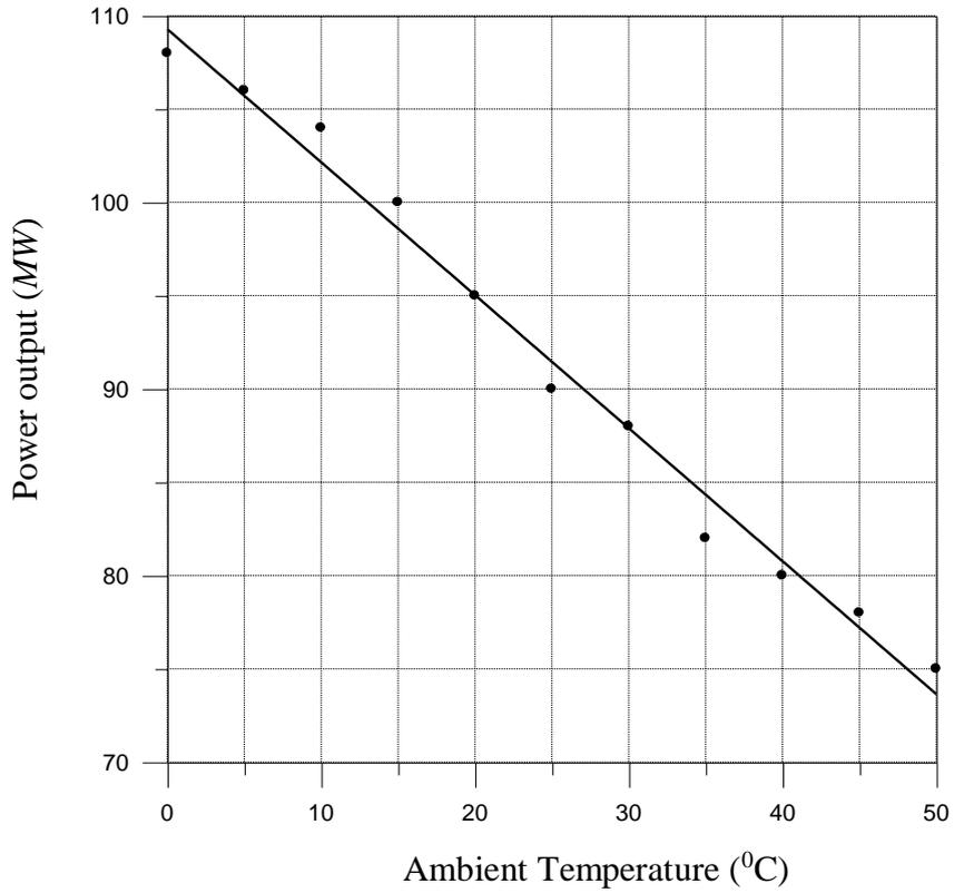
**Figure (4):** Ambient Temperature versus output Power
