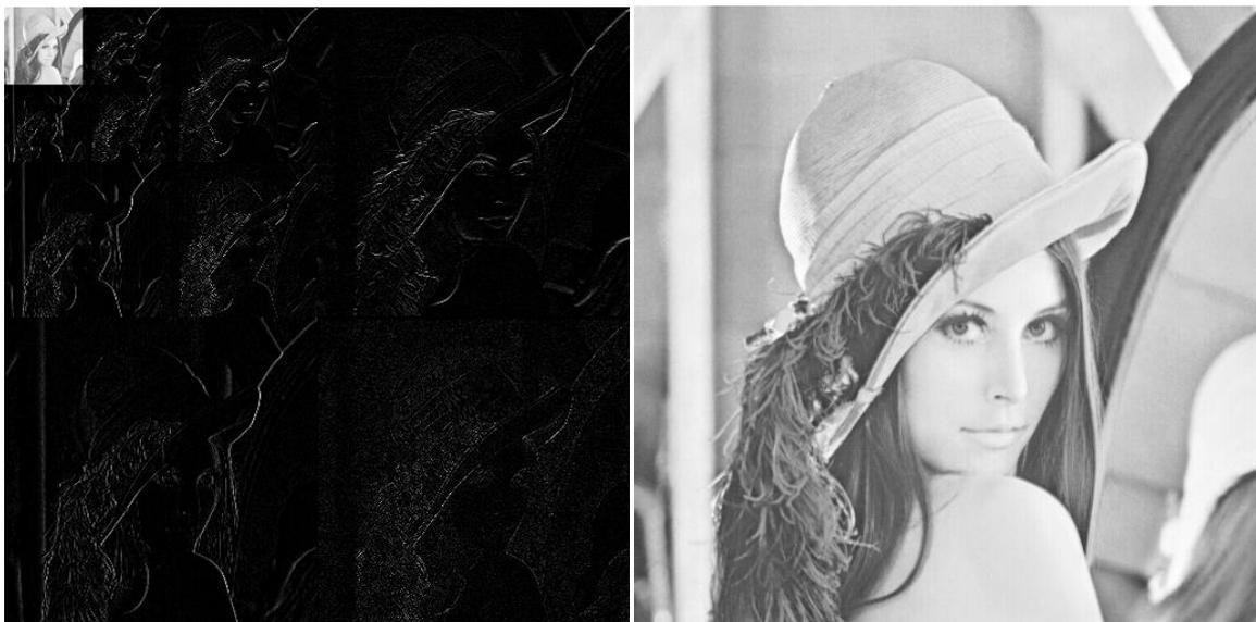
**Figure (3):** Three-level DHWT decomposition of Lena image and its reconstructed version.
