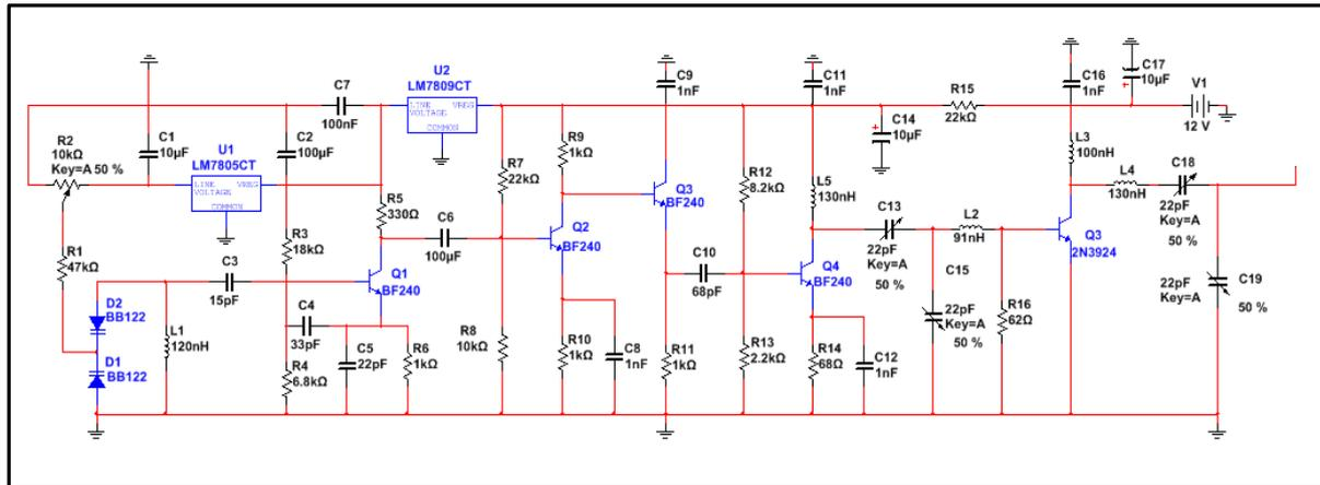
**Figure (2):** The 416MHz Signal Transmitter.
