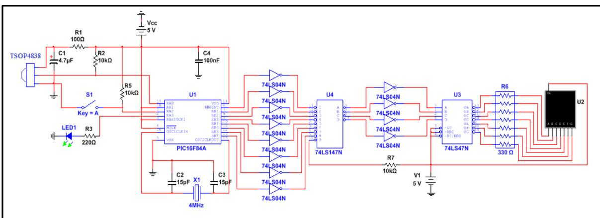
**Figure (4):** The Electronic Circuit of the Laser Decoder.
