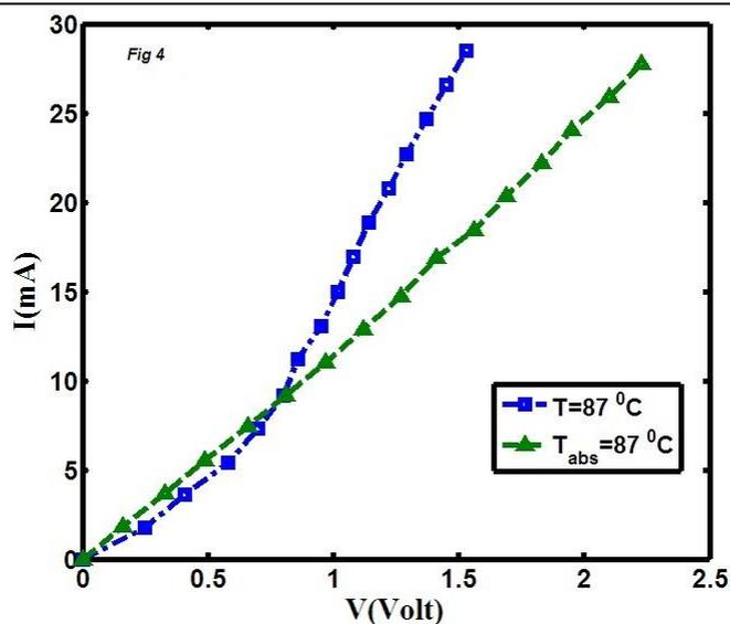
**Figure 4:** I-V diagram for carbon nanoparticle at 87 °C in either gas adsorption or lack of gas adsorption.
