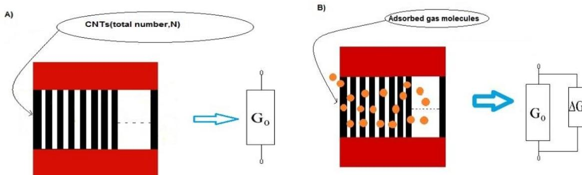
**Figure 1:** A: Sensor before the gas adsorption, B: Sensor after the adsorption of gas molecules
