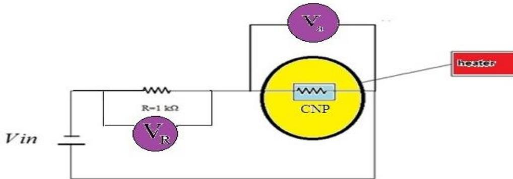
**Figure 2:** The circuit for the carbon nanoparticle electrical resistance measurement.
