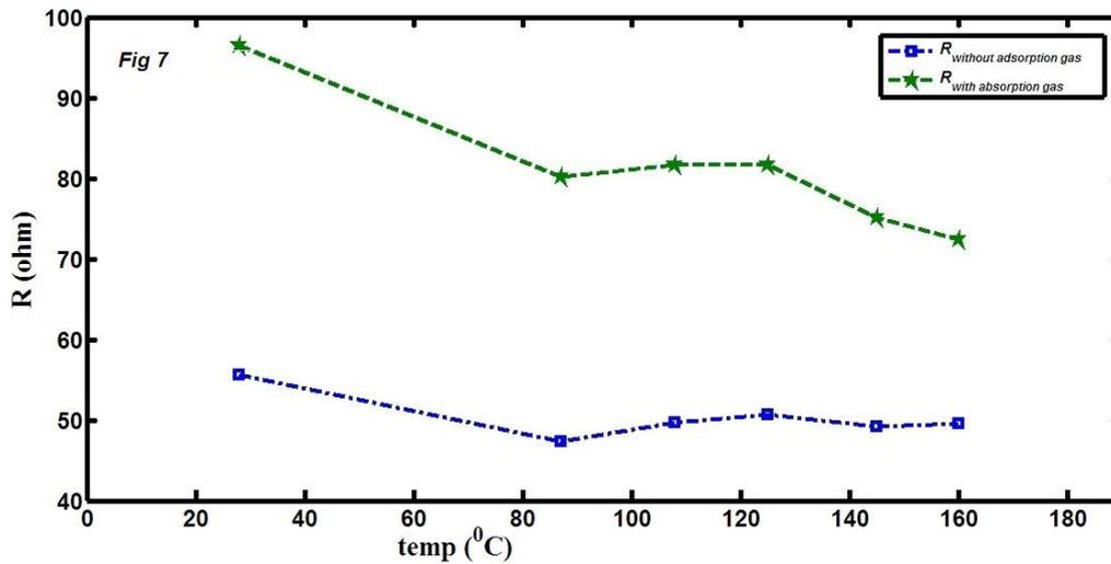
Figure 7: Resistance vrsuse temperature in the precence of gas(green line) and without gas,(blue line)
