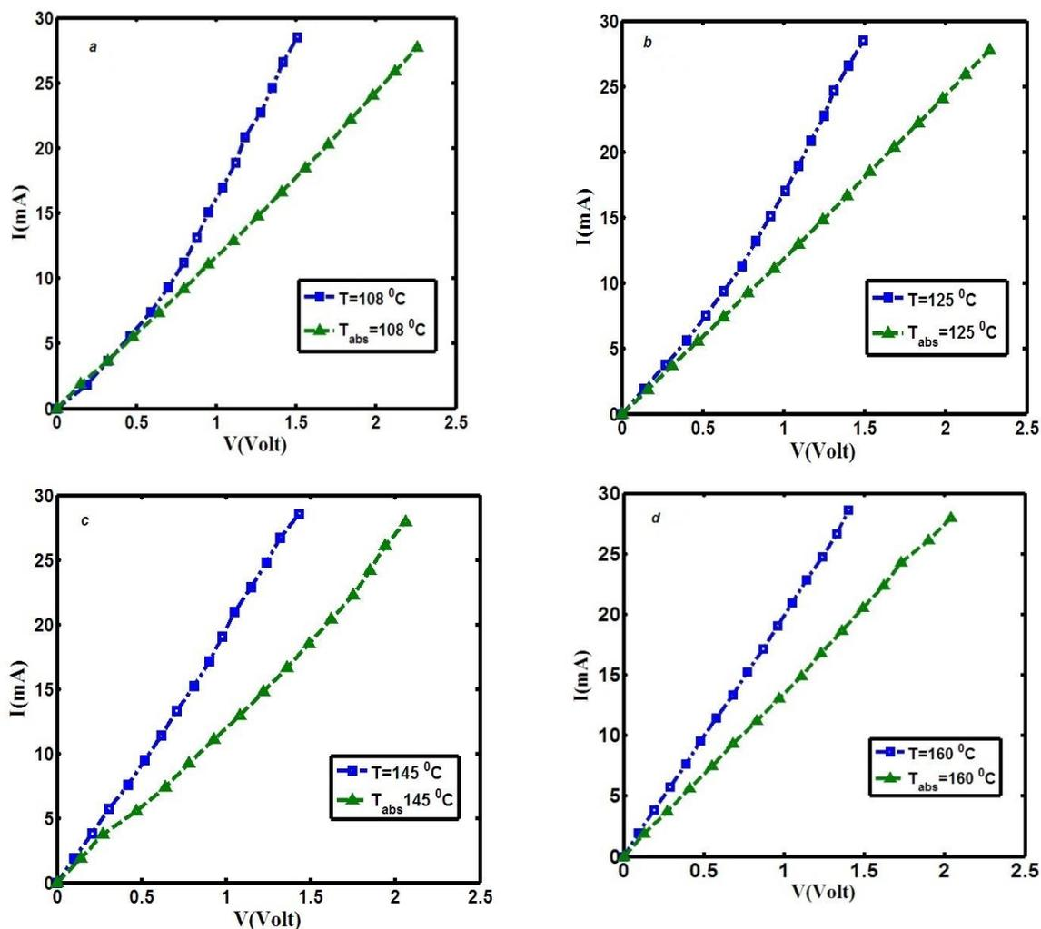
**Figure 5:** a). I-V diagram for carbon nanoparticle at 108 °C, b). at 125°C, C).at 145°C, d).at 160°C in either gas adsorption and without gas respectively.
