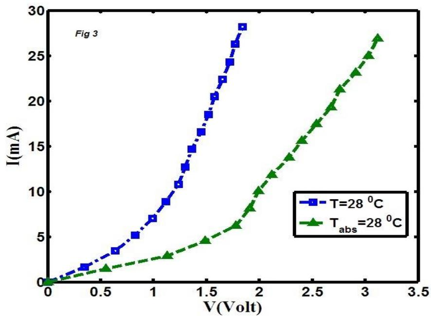
**Figure 3:** I-V diagram for carbon nanoparticle at  $28^\circ\text{C}$  in both gas adsorption and lack of gas adsorption.
