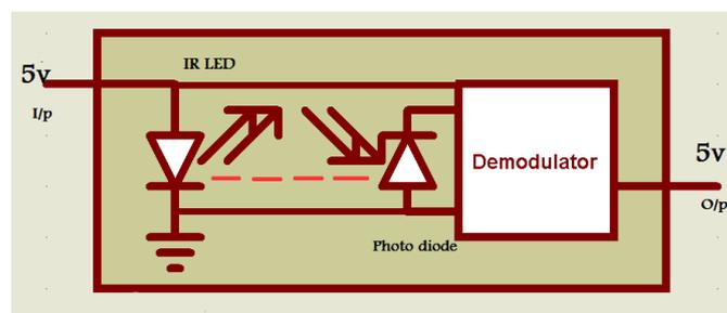
Figuer.2: Remote Sensing Circuit
