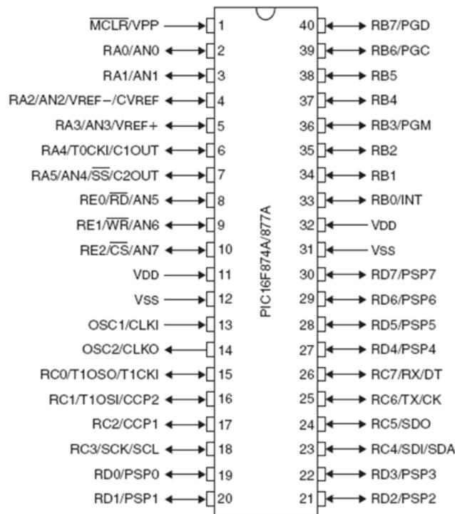
**Figuer.4:** PIC16F877A Microcontroller
