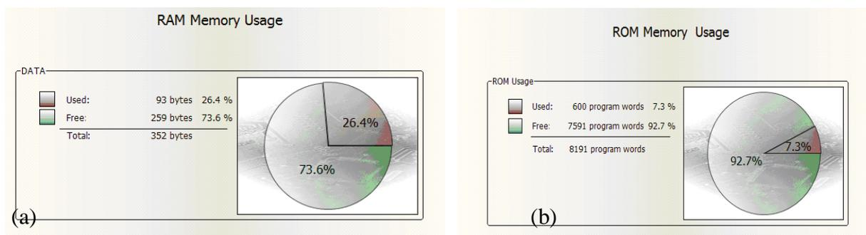
**Figuer.9:** Memory Graph used in PIC, (a) RAM, (b) ROM
