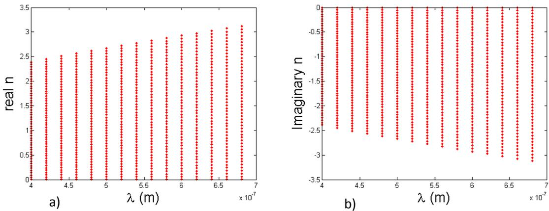
**Figure (5):** a) The wave length increment effect on real part of refractive index b) The wave length decrement effect on imaginary part of refractive index in degenerate condition with applied bias
