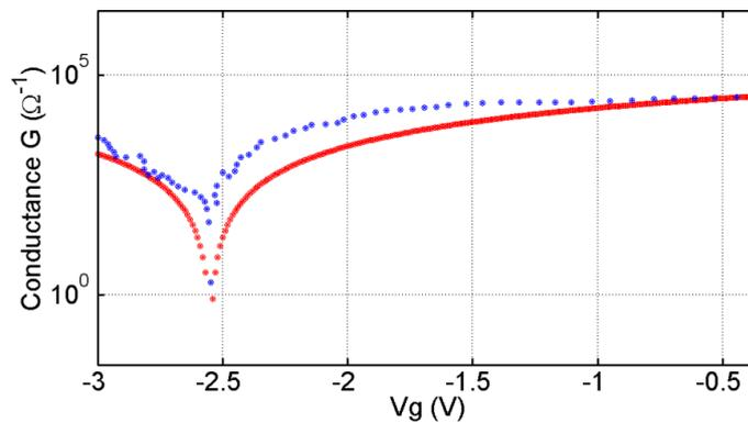
**Figure (2):** BGN conductance model in comparison with experimental data [24]
