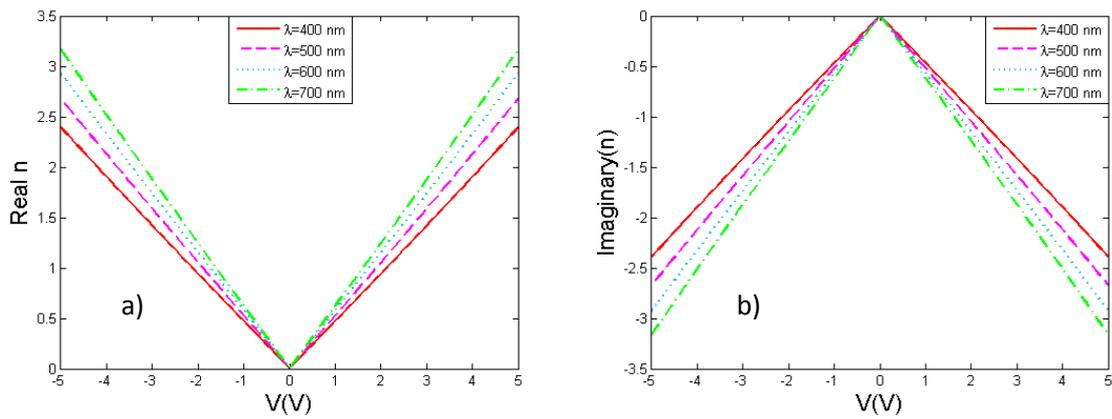
**Figure (4):** a) Applied bias effect on real part of refractive index b) Applied bias effect on imaginary part of refractive index both for different wave lengths
