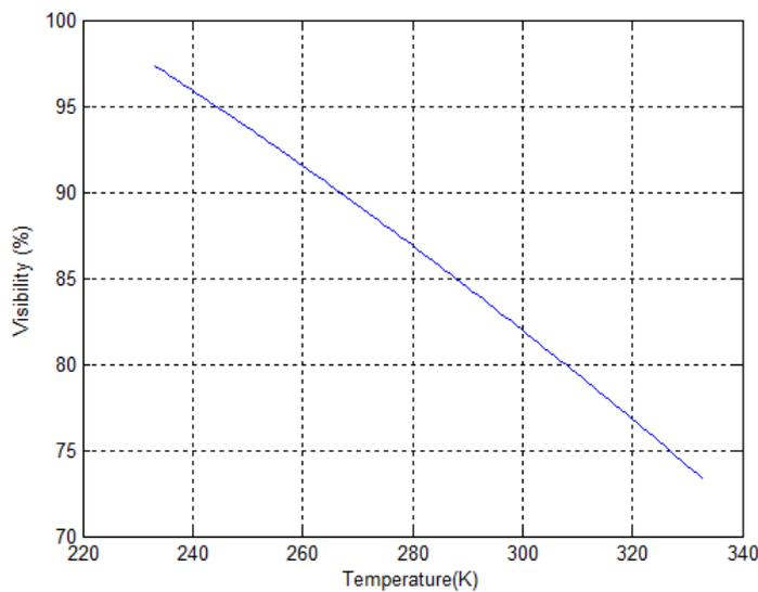
**Fig. (3):** The effect temperature on the visibility of MZIM (233 – 333) K
