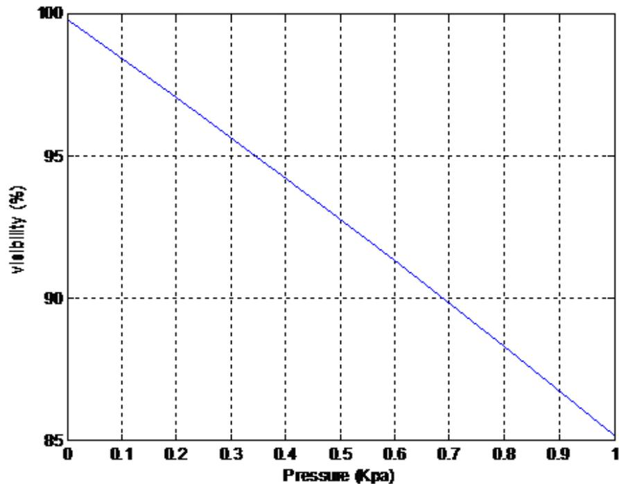
Fig. (10): The effect pressure on the visibility of MZIM (223 K) (0 - 40 Kpa)
