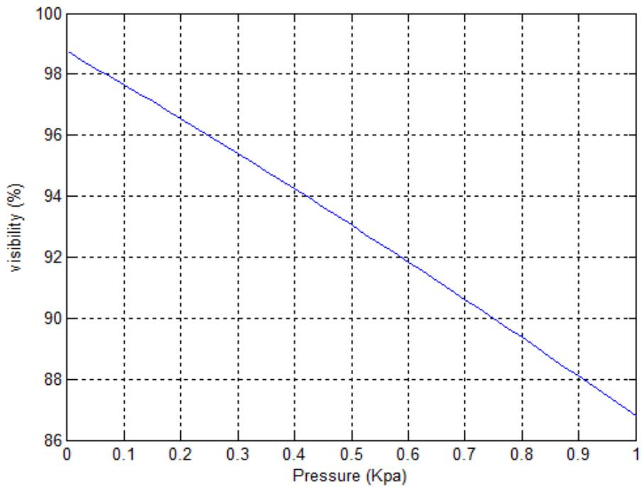
**Fig. (8):** The effect pressure on the visibility of MZIM (293 K) (0 - 40 Kpa)
