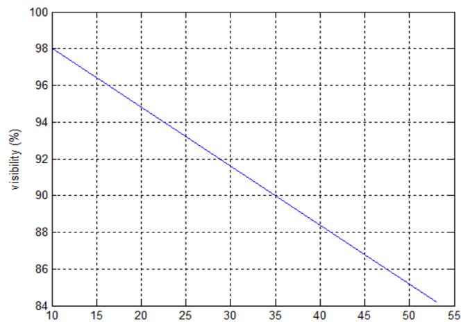
**Fig. (6):** The effect strain on the visibility of MZIM (258 K) (10 - 55  $\mu\epsilon$ )
