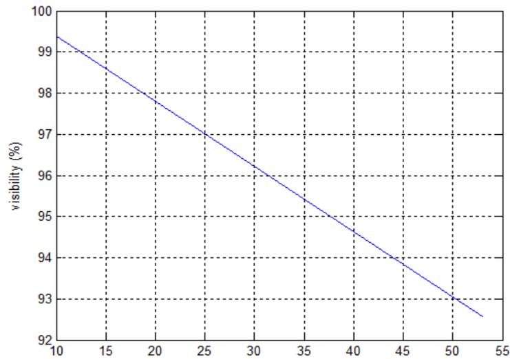
**Fig. (4):** The effect strain on the visibility of MZIM (333 K) (10 - 55  $\mu\epsilon$ )
