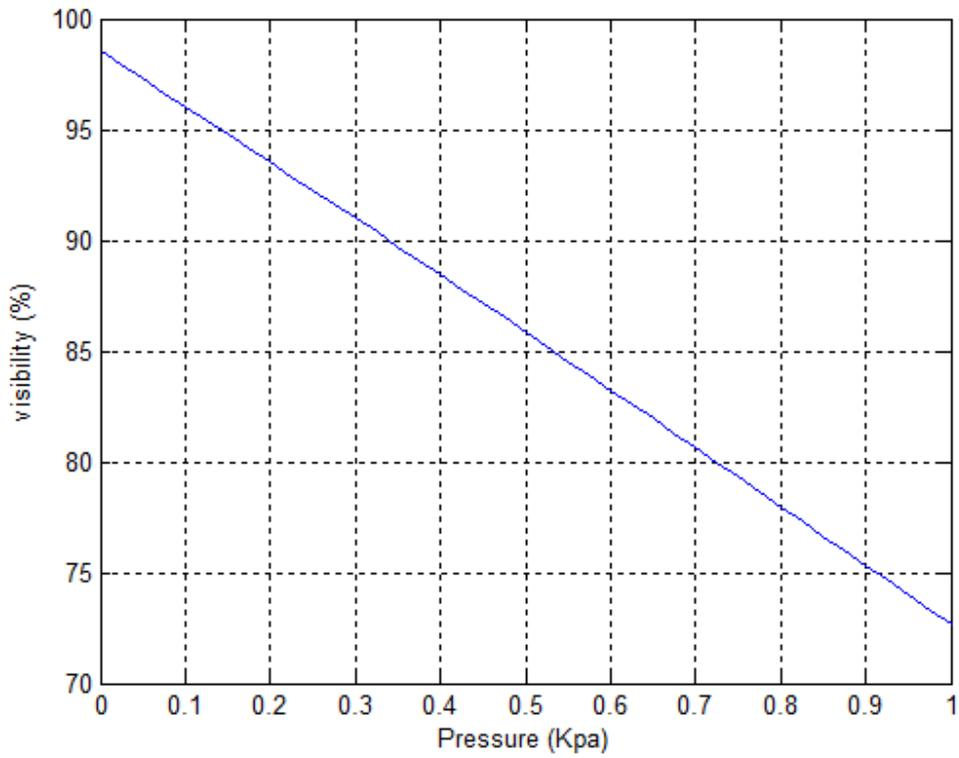
**Fig. (7):** The effect pressure on the visibility of MZIM (323 K) (0 - 40 Kpa)
