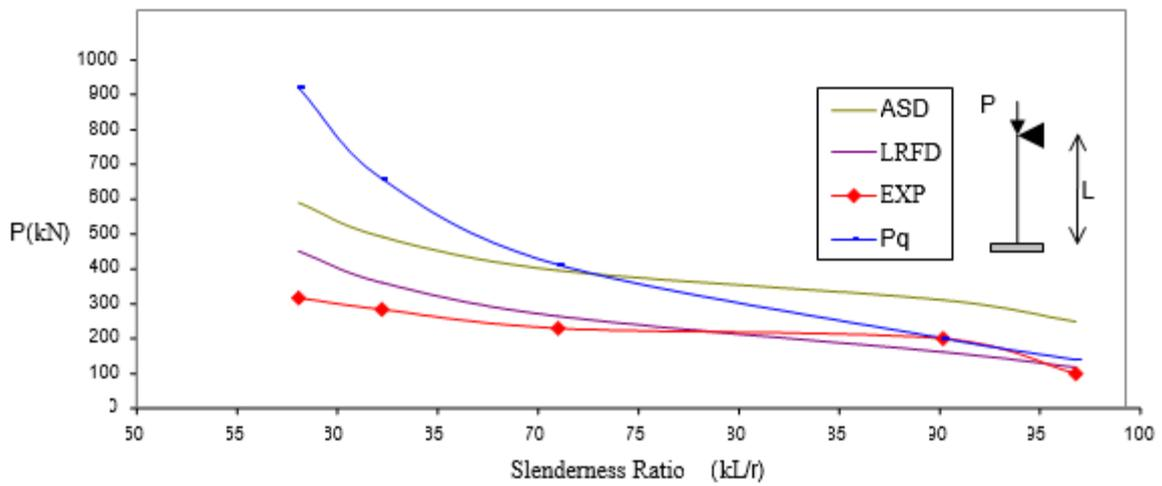
**Fig. (4):** Comparison between Theoretical and Experimental Loads for Propped Cantilever.
