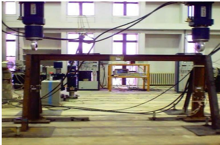
**Fig. (2):** Test Rig setup (steel portal frame IPE section subjected to two concentrated loads)
