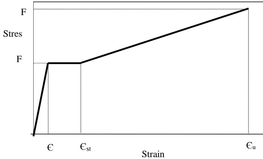
**Fig. (1):** Idealized Stress-Strain Curve derived from experimental tensile tests.
