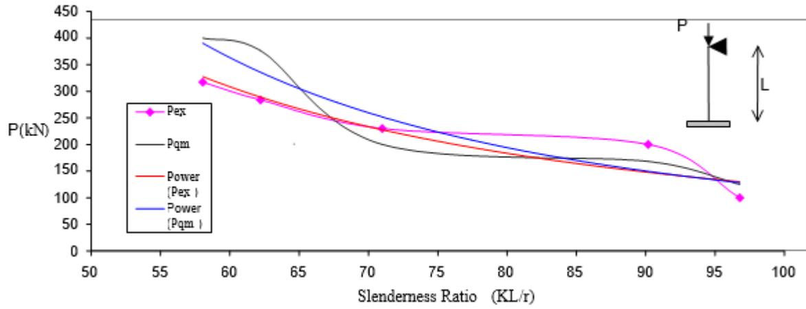
Fig. (6): Comparison between Quasilinear and Experimental Loads (Material Nonlinearity).
