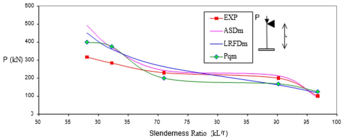
**Fig. (5):** Comparison between Theoretical and Experimental Loads (Material Nonlinearity)
