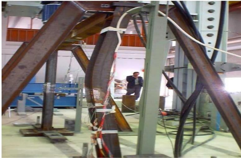
**Fig. (3):** Column Failure due to Buckling in Minor Axis mode Bending
