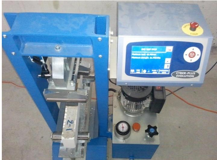
Figure 7.A specimen in compression machine
