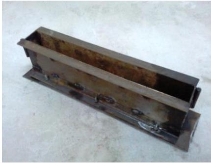
Figure 1. Typical steel mold
