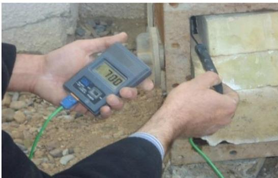
Figure 5. Digital thermometer used
