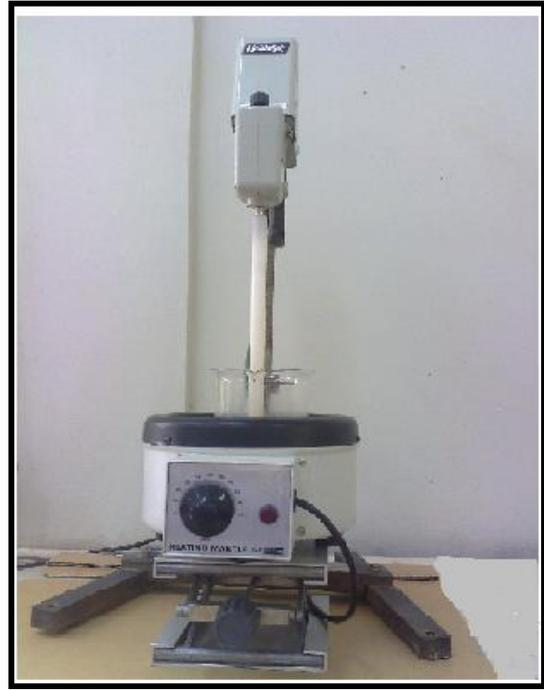
**Fig (2):** Mechanical stirrer with controller of temperature of heating path using in catalysts preparation.
