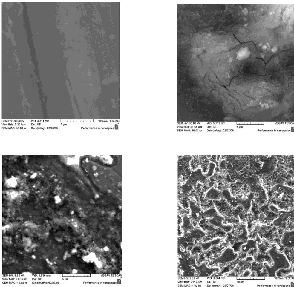
**Fig. (4):** SEM morphology of the anodic surface: (a) polished Surface (b) 10 min. Anodizing (c) 20min. Anodizing (d) 30min. Anodizing
