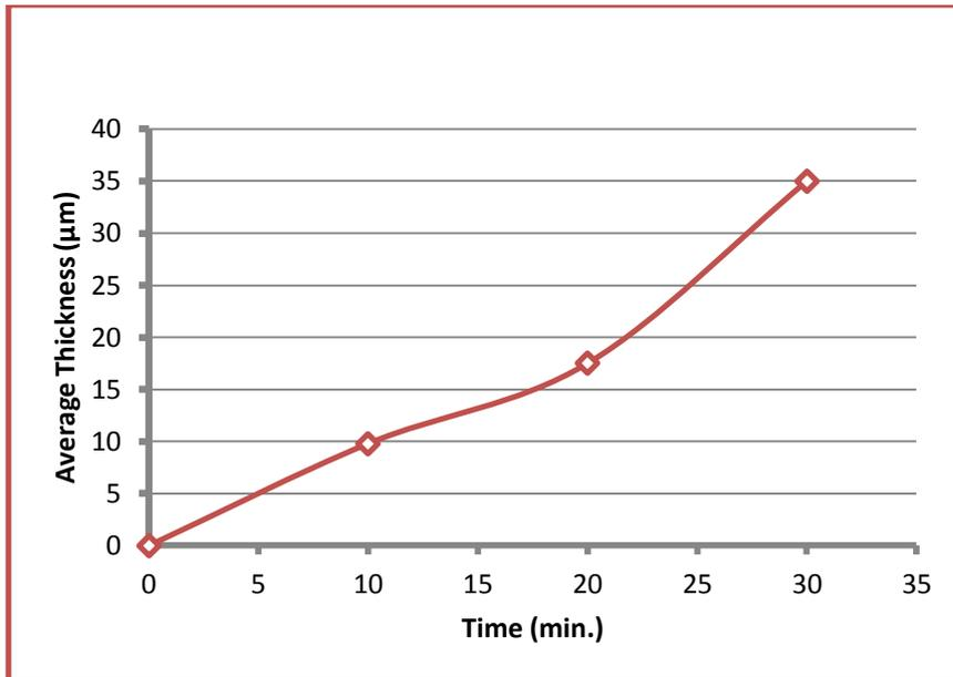
Fig (5): Variation of coating thickness with anodizing time
