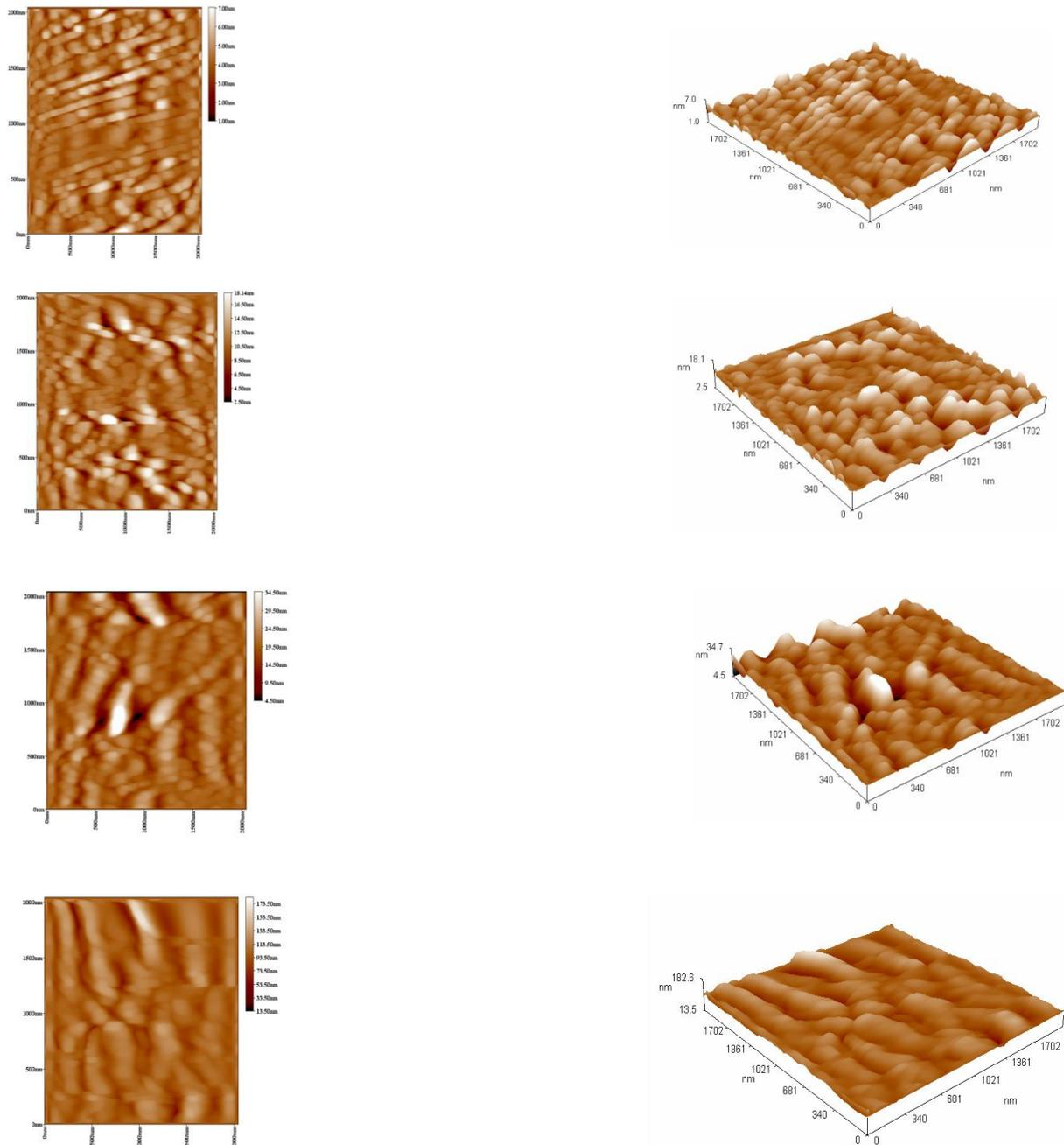
**Fig (2):** 2D and 3D AFM images for Mg AZ31 Alloy (a) polished Surface (b) 10min. Anodizing (c) 20 min. Anodizing (d) 30 min. Anodizing
