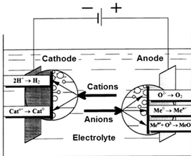
**Fig (1):** Electrode Processes in aqueous solutions <sup>(9)</sup>
