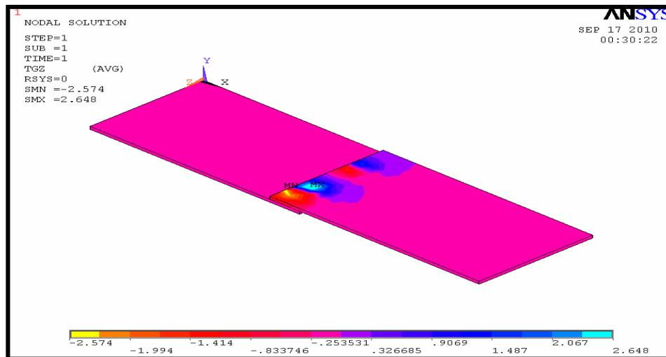
Fig. (10): Total temperature gradient in laser welding process.
