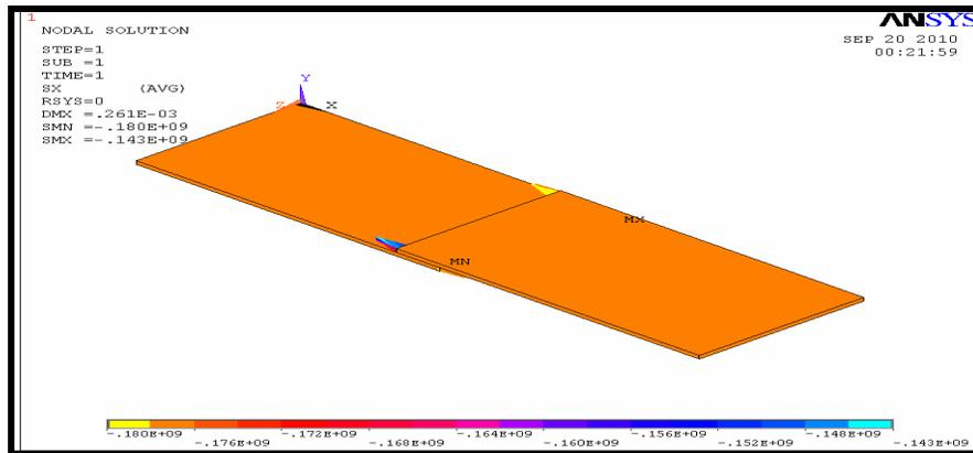
Fig. (8): ANSYS -11 stress distribution in x-direction.
