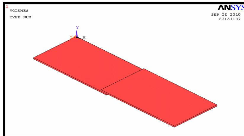
Fig. (3): Two piece of metal lap positioned to be welded.
