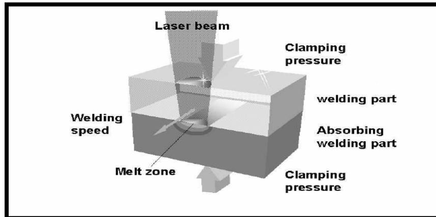
Fig. (2): Laser beam welding process <sup>(4)</sup>.
