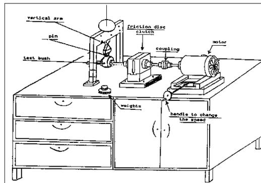
**Fig.(2):** Wear Test Machine .
