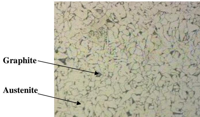
**Fig.(9):** Microstructure of welding zone (Mag. X65).
