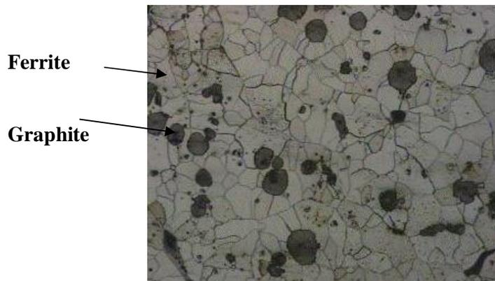
**Fig. (7):** Microstructure of nudulare cast iron (Mag.X 65).
