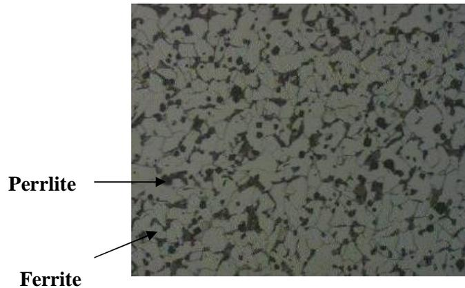
**Fig.(8):** Microstructure of nudulare cast steel (Mag. X130).
