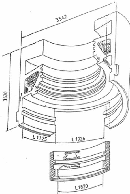
**Fig. (1):** Steam turbine inner case (dimensions in mm).
