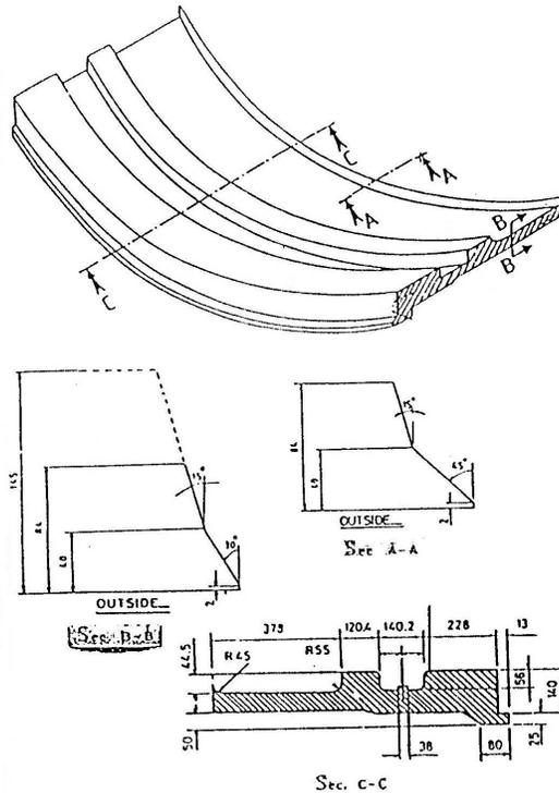
**Fig.(3):** Compensated cast steel with joints preparation.
